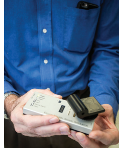
LEFT: THE RADIO TRANSMITTER USED TO INTERFACE WIRELESSLY WITH THE MONKEY BRAIN
